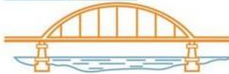
tied arch bridge
